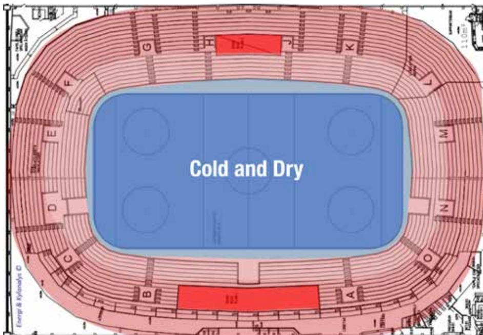
One of these examples is Scaniarinken, an ice hockey stadium in Sweden with capacity of 6200 spectators. Before interventions there was a temperature difference of 8°C between the top and the bottom of the stands. Nowadays, this temperature difference is reduced to less than 2°C only.
