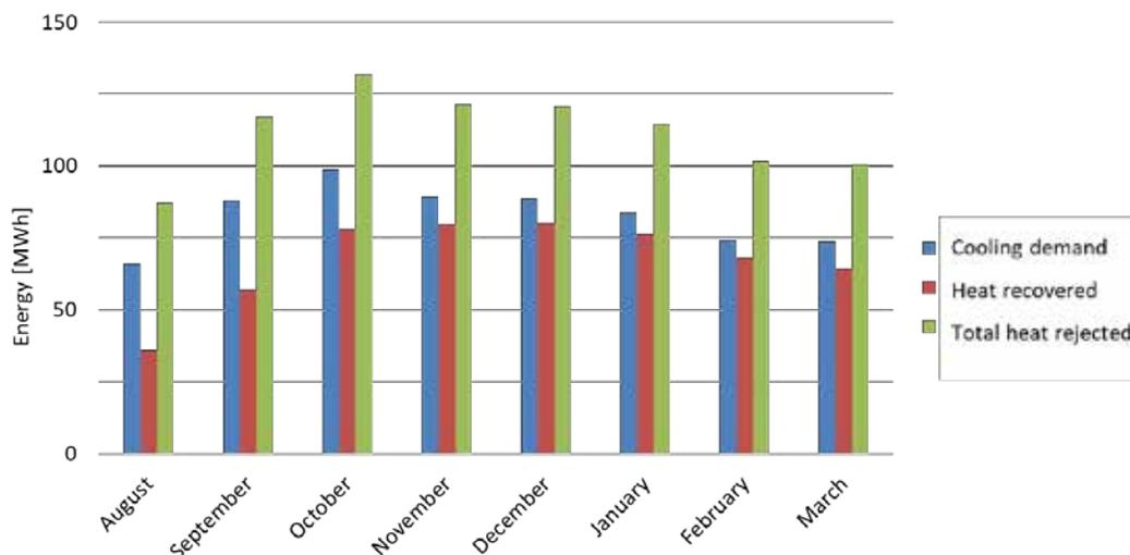
**Figure 26.** The refrigeration system usually releases more heat than what a typical ice rink needs. It is therefore interesting to look for heating demands beyond an ice rink.
