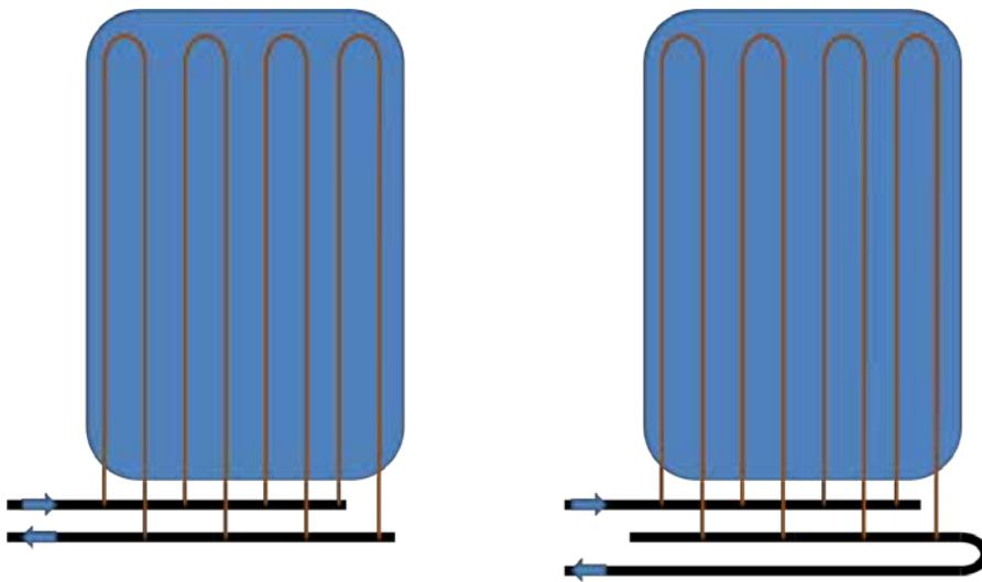
**Figure 19.** Two different header arrangements: conventional (left) and reversed return (right), where the latter is generally recommended.
