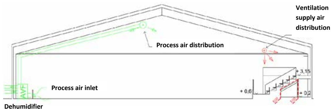
**Figure 45.** Air supplied to different zones in ice arena: Dehumidified air above the ice, and heated air towards the stands. Fresh air intake only when necessary.
