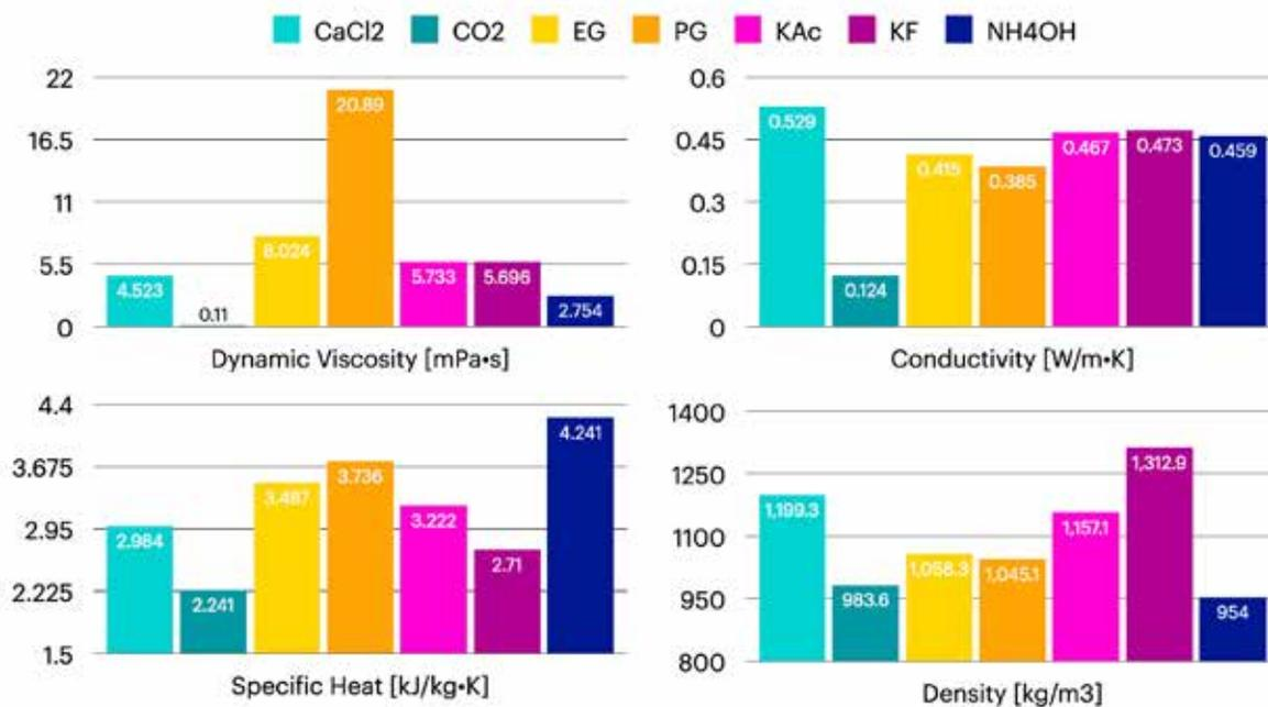
Figure 31. Thermophysical properties of discussed secondary refrigerants at -10°C having freezing points of -20°C (Kilberg, 2020).
