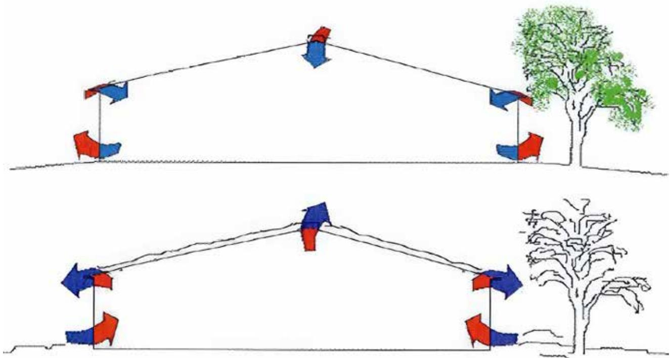
**Figure 12.** Stack effect in an ice rink depending on a time of a year (Rakennustieto, 2007)
