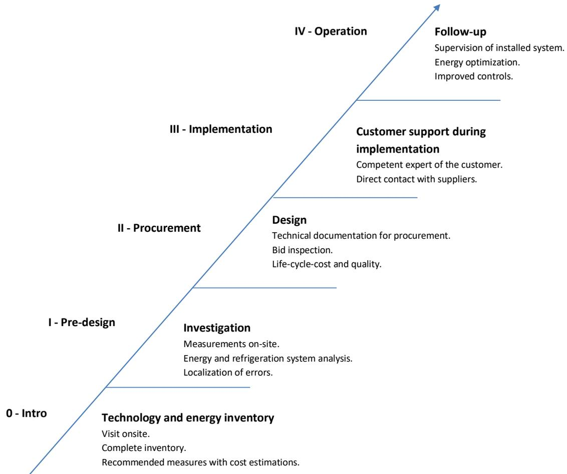
In the illustration above, the work process of developing energy concepts is shown for newly built or to be renovated ice rinks, in order to optimize the facility or lower its operating costs. Different arenas have different requirements; therefore, every ice arena needs a tailored solution.
