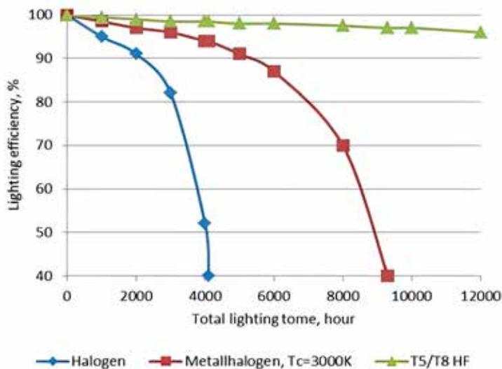
**Figure 52.** Efficiency of different lighting types during their lifespan.
