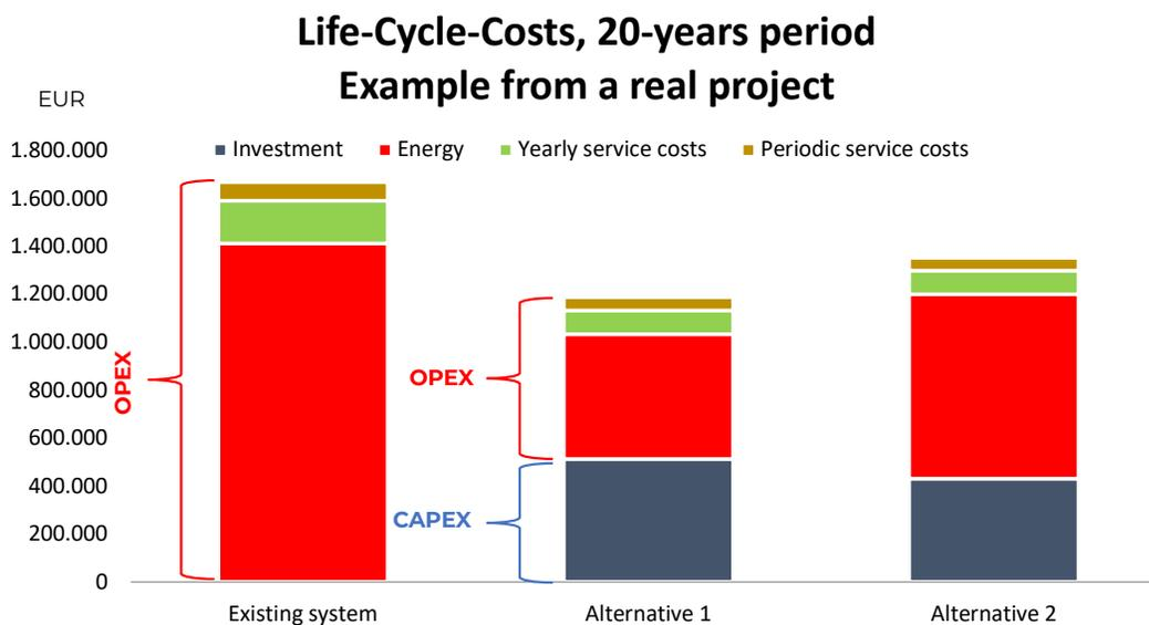
**Figure 6.** Life-cycle cost results for sustainable energy solutions (alternative 1 & 2) in an ice rink compared to existing system. The results show that investing in long-term solutions will yield the biggest savings for the ice rink owner.
