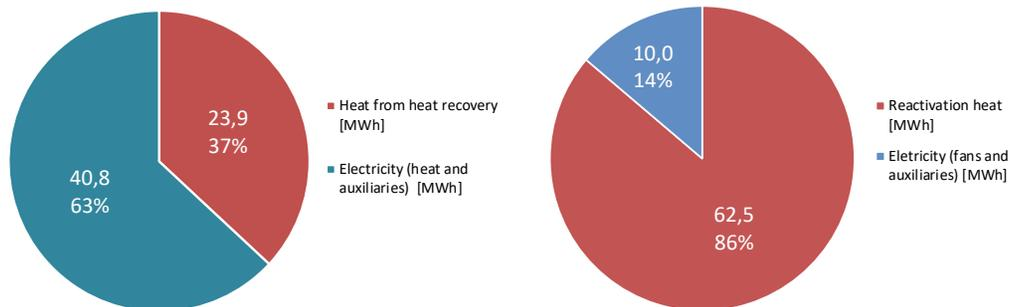
**Figure 44.** Application of recovered heat from a modern refrigeration system in the reactivation process leads to energy savings of ca 40% in Gen 1 and 85% in Gen 2 sorption dehumidifiers.
