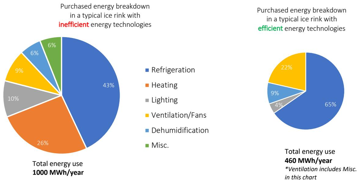
**Figure 4.** Main energy uses in a typical/conventional ice rink in Sweden with inefficient and efficient energy technologies (Stoppsladd, 2014; ASHRAE, 2017).
