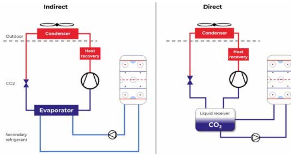
**Figure 28.** Principle of a CO2 indirect to the left and CO2 DX to the right, with heat recovery.
