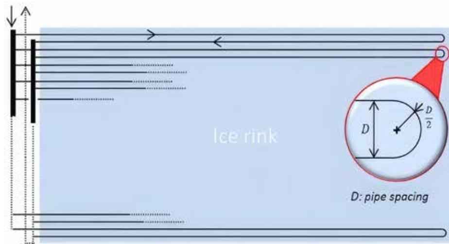
**Figure 18.** Typical piping layout in Europe with headers on the one short end side.
