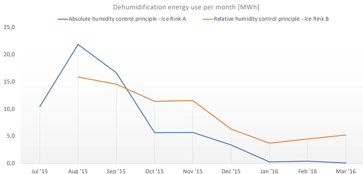
**Figure 43.** Comparison of energy use between control strategies based on relative humidity and dewpoint/absolute humidity in two ice rinks.
