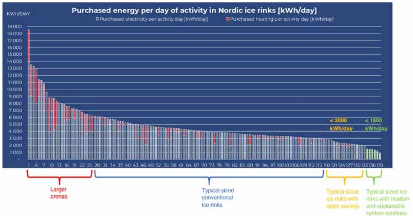
**Figure 5.** Comparison of energy performance in Nordic ice rinks. The shown values reflect the average amount of purchased energy (electricity and any other potential heat source) during a day of ice arena activity.
