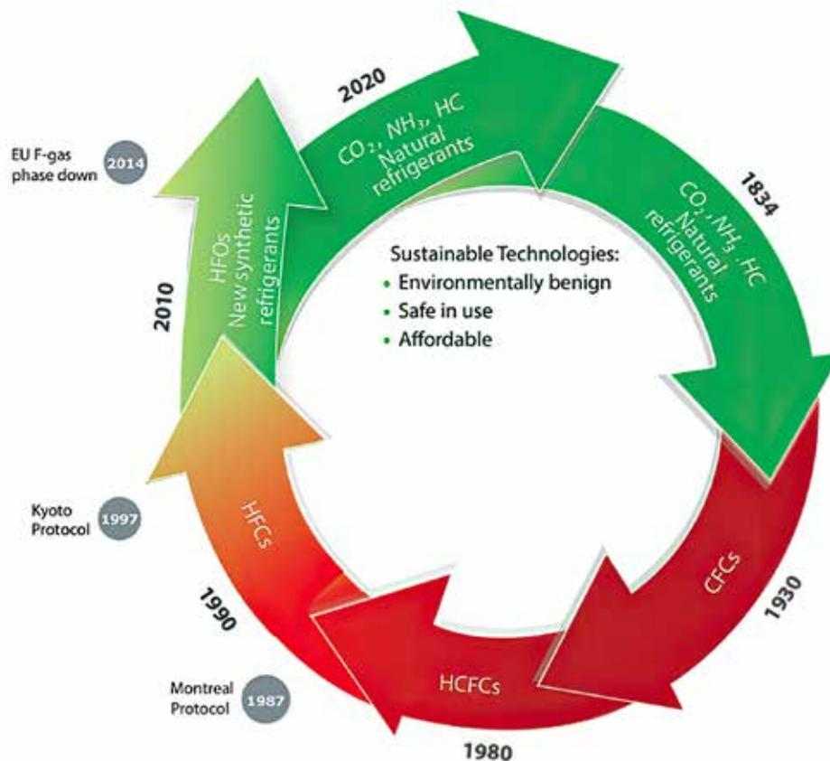
**Figure 24.** The global tendency is to “return to the roots” and select natural refrigerants (Danfoss).
