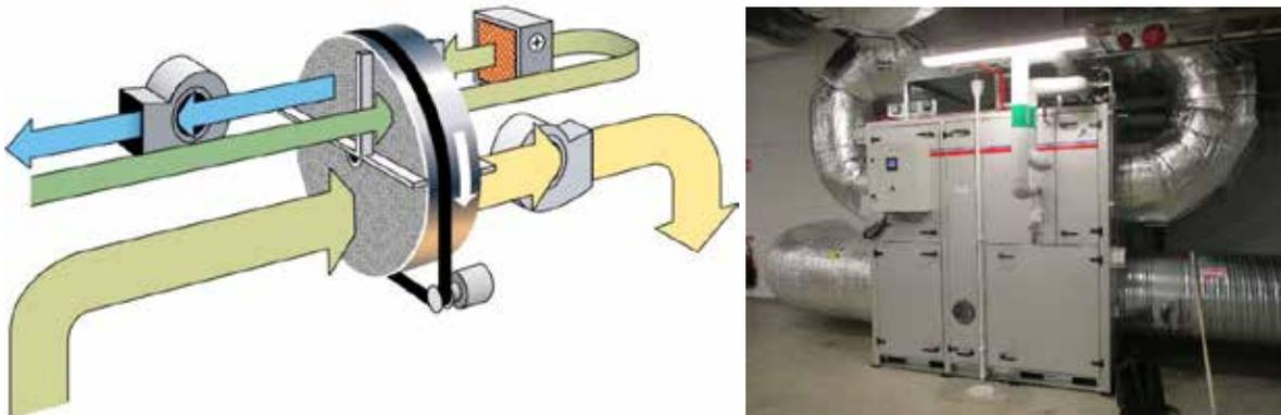
**Figure 40** The working principle of a sorption type of dehumidifier (left) and unit (right).
