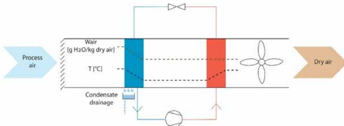
**Figure 41** The working principle of a refrigeration type of dehumidifier.
