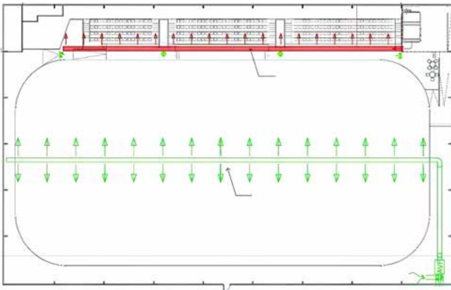
**Figure 46.** The ventilation and dehumidification distribution systems should be separated.
