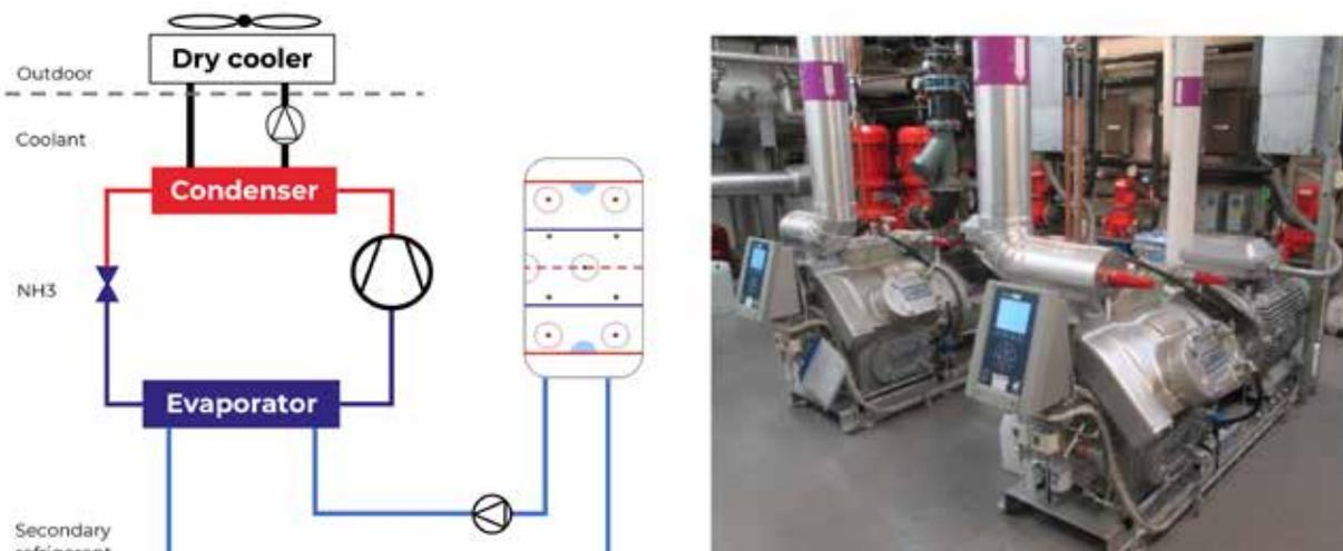
**Figure 30.** A modern fully indirect NH<sub>3</sub> refrigeration system.
