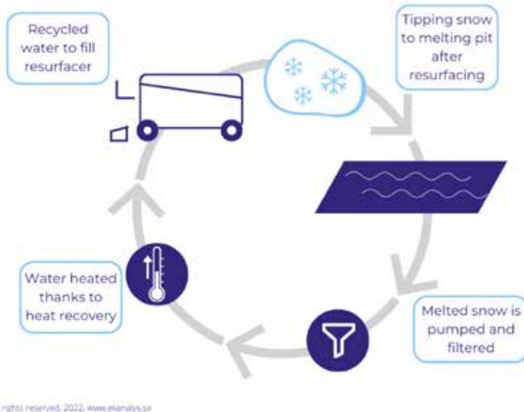
**Figure 59.** Water recycling applied in melting pit function.
