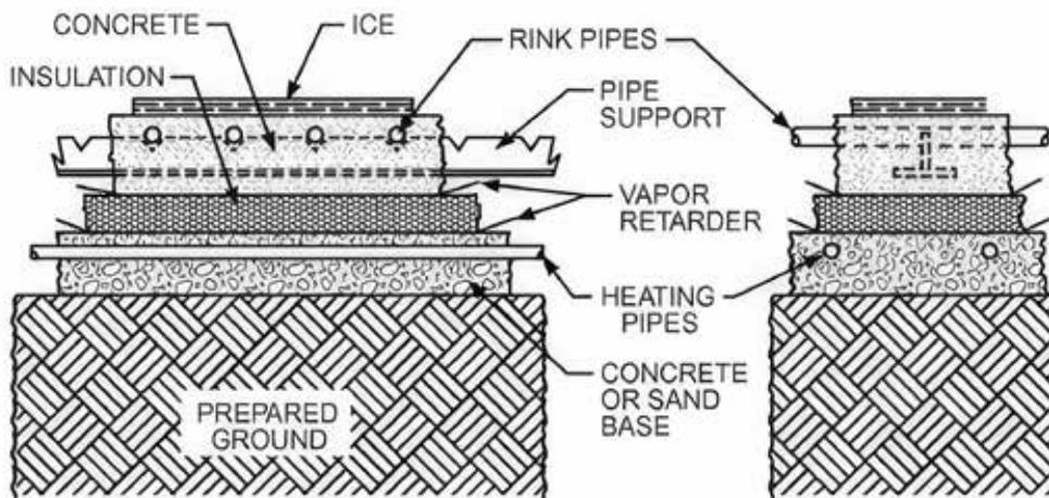
**Figure 17** Typical layout of and ice rink floor (ASHRAE Refrigeration, 2014)
