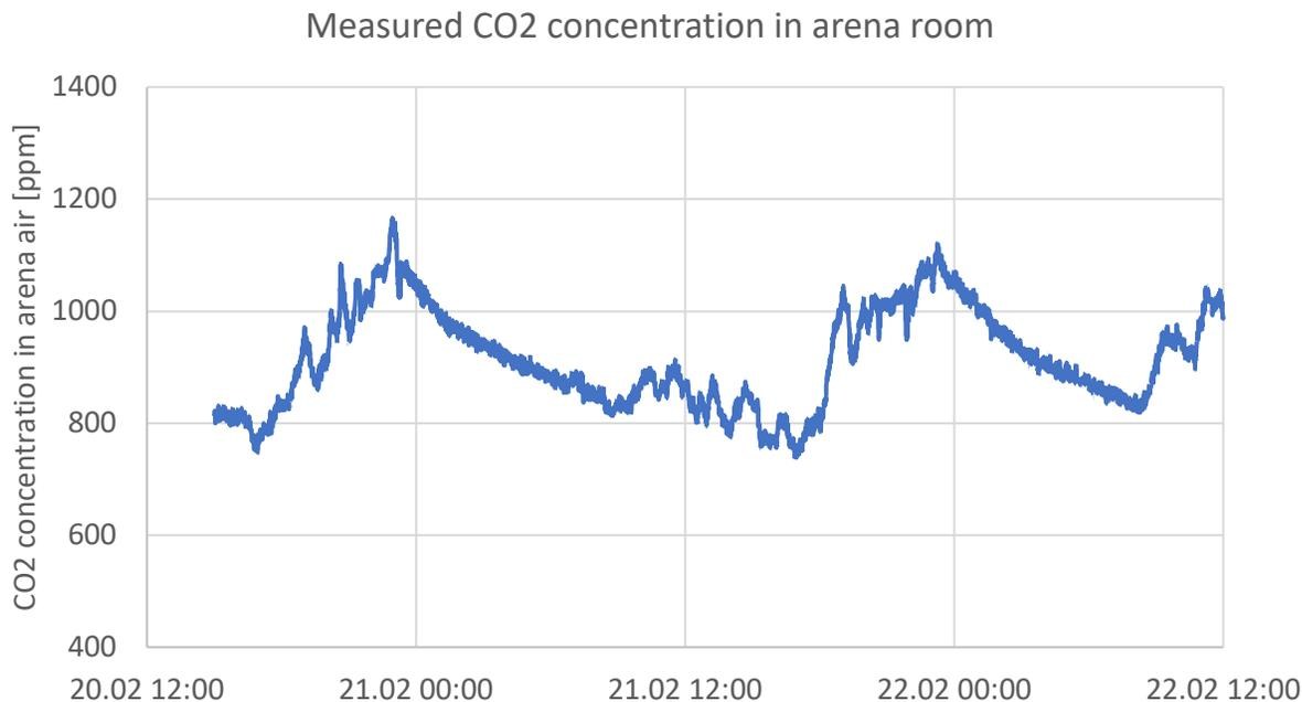
**Figure 50.** Measured CO<sub>2</sub>-levels in a typical Nordic ice rink operating on full air recirculation.
