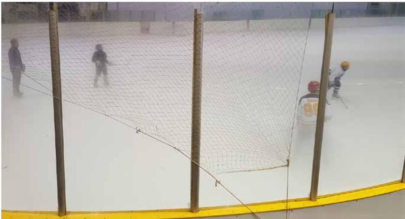
**Figure 2.** A well-functioning ice arena must be able to handle the complex heat loads and moisture loads that come along with this specific environment. In this picture they are not well managed, causing foggy conditions.
