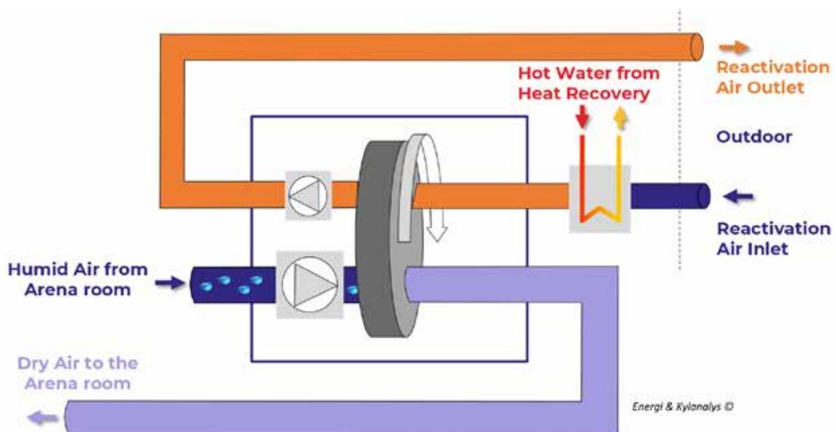
**Figure 42.** Sorption based dehumidification that utilizes the heat recovery from refrigeration, referred to as Generation 2.
