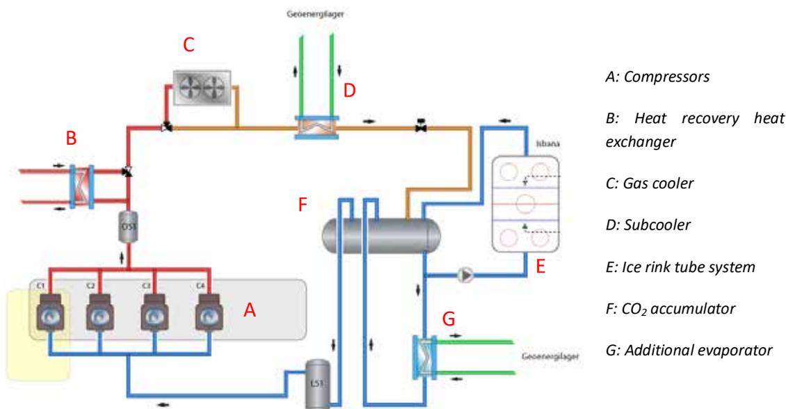
**Figure 29.** Overview of a CO<sub>2</sub> DX refrigeration system in an ice rink.
