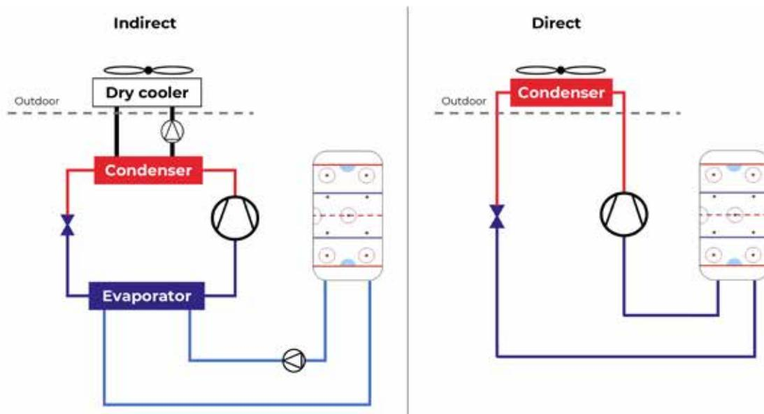
**Figure 23.** Two main refrigeration system configurations in ice rinks, simplified schematic.
