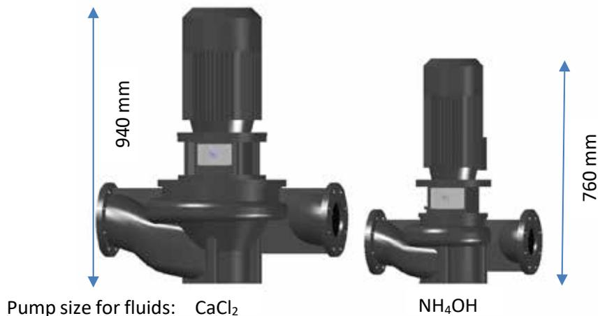
**Figure 34.** Required pump size difference between  $\text{CaCl}_2$  pump (on the left) and  $\text{NH}_4\text{OH}$  pump (on the right), for the same cooling capacity of 250 kW at  $-10/-8^\circ\text{C}$ .
