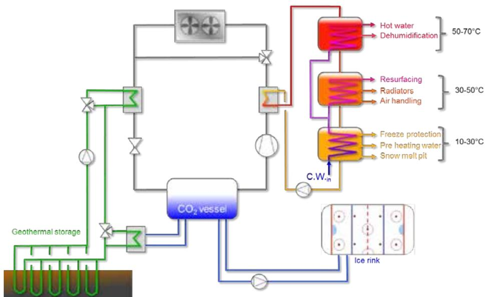
**Figure 38.** Principle overview of a refrigeration and heat recovery system (Illustration by EKA).
