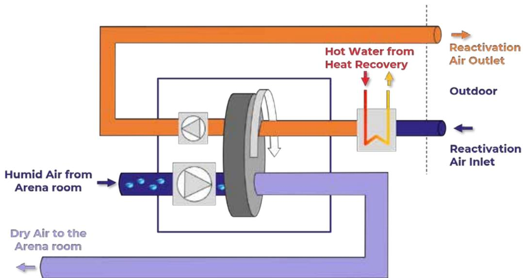
Heat recovered from the refrigeration cycle can be utilized for dehumidifying the air. In the sport facility called Testebo, Sweden, the solution was implemented where ca 85% of the energy cost for dehumidification can be covered by the heat recovery. The estimated energy saving is equivalent to 5000 - 6500 Euros/year.
