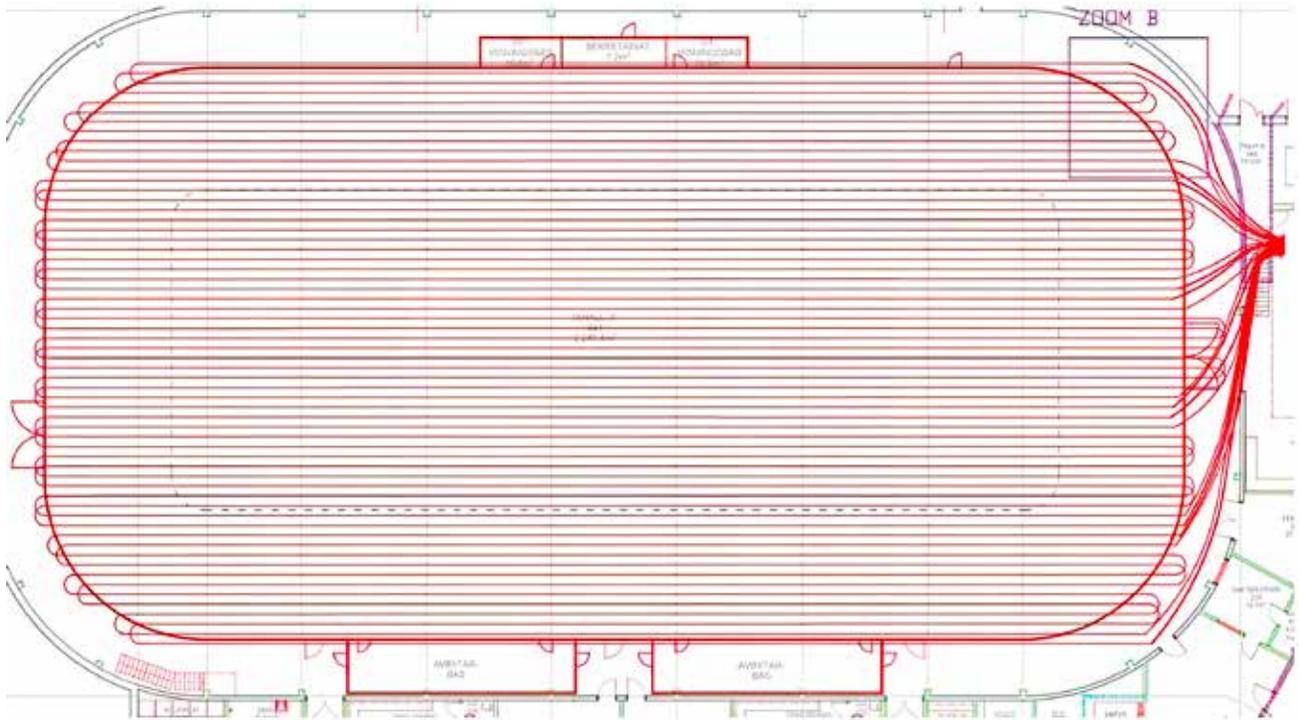
**Figure 20.** Principle solution on freeze protection distribution below the rink floor.
