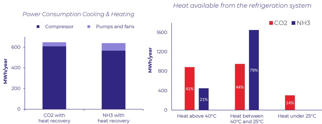
The aim of the study was to identify the best solution in terms of system layout and refrigerant. The calculation shows that difference in terms of power consumption between CO2 and ammonia is negligible.
